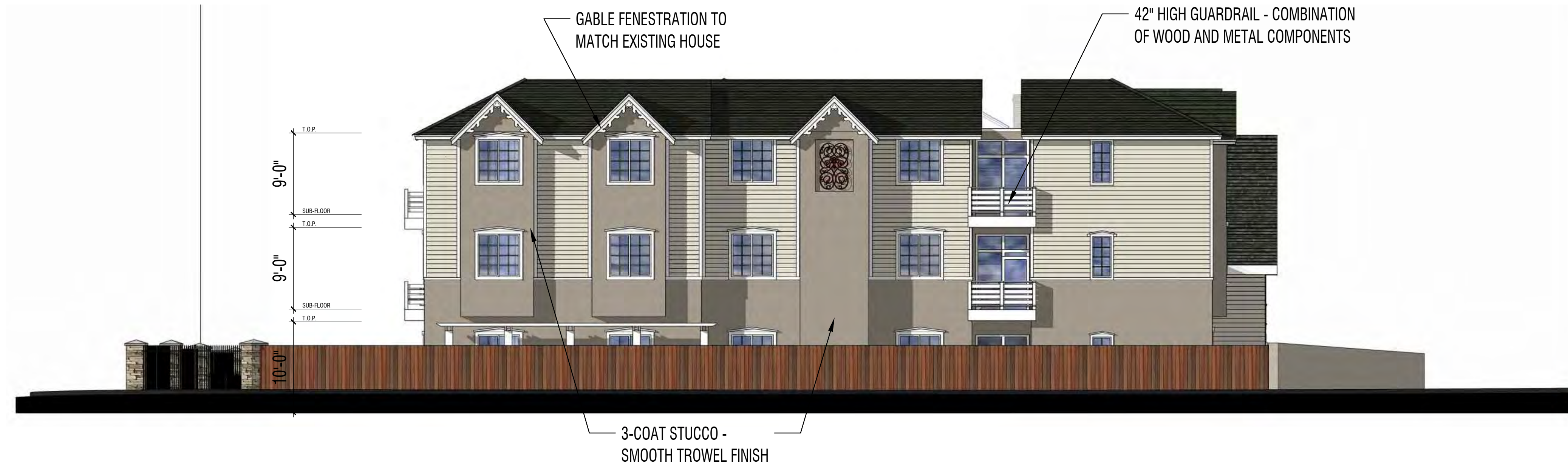
WEST ELEVATION (RIGHT SIDE)
